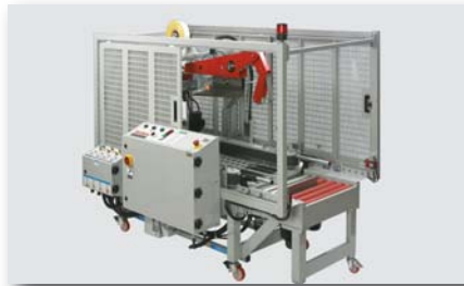
800rf – Fully automatic for consistent flow and sealing without an operator. Automatically adjusts for random sizes, folds top minor and major flaps and seals up to 10 cases/minute. Includes up to 48 mm wide tape.
