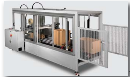
2000rf – For a high volume with random case sizes or where different lines converge for sealing. Fully automatic 3-stage operation separates, folds, and seals tops and bottoms at up to 20 cases/minute. Uses 36 mm to 48 mm tape widths.
